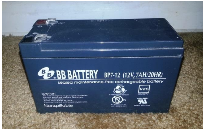
Figure 54: A lead-acid battery removed from a motorcycle
