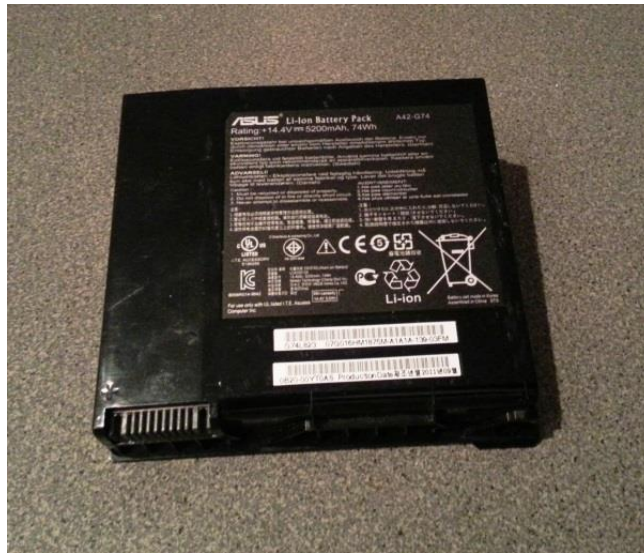
Figure 57: A 14.4V Li-ion battery that we removed from an Asus notebook.
