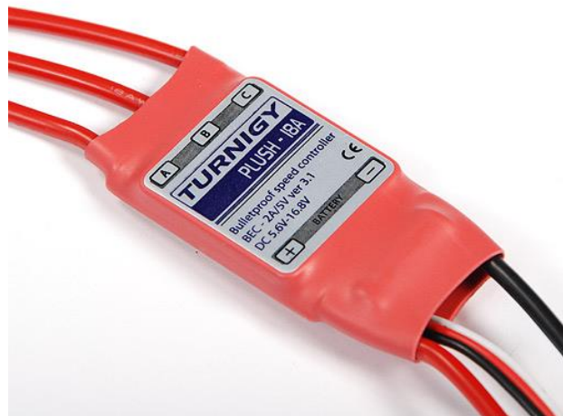
Figure 64: The 18A Turnigy Plush Electronic Speed Controller we decide to use in our prototype (permission pending)
