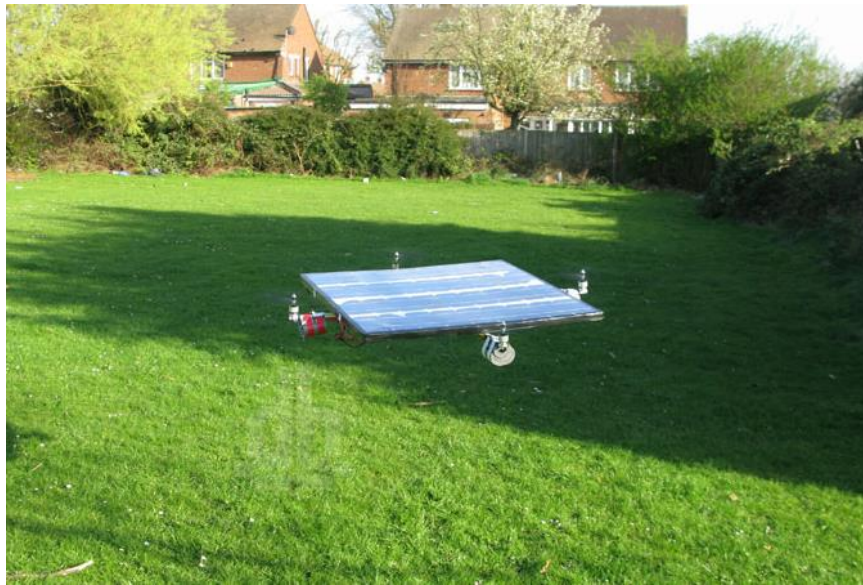
Figure 52: A solar-powered quadcopter built by master's students at Queen Mary University of London Permission Pending.
