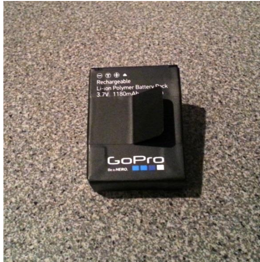
Figure 58: A 3.7V Li-Po battery that we removed from a GoPro camera
